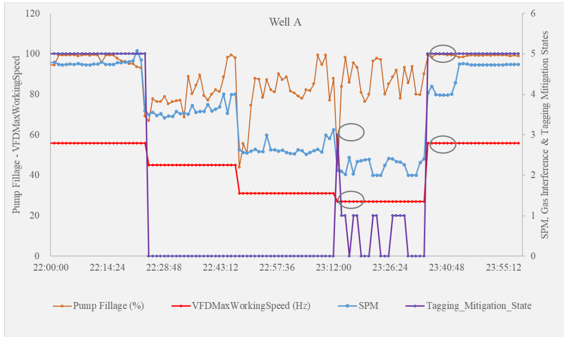
Figure 6: Speed control by edge gateway utilizing the tagging mitigation algorithm.
