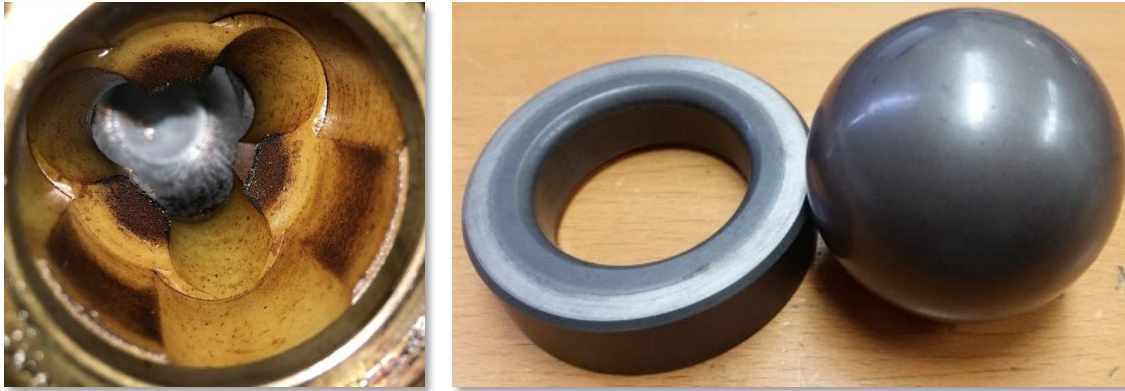
Figure 6 – Typical IR Cage inspection. The cage material has some minor surface discoloration, but this does not affect its performance. The material is inspected, specifically around the tabs and ball guides and determined to be fully functional. Balls and seats are assessed through the usual vacuum test process. In all of the above Case Studies, the cage and ball/seat were assessed to be in good condition and re-deployed as-is.
