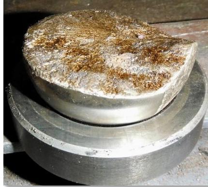
Figure 4 – Ball and seat issues are not always attributed to cages. The ball impacts both the seat and the cage and so it sees twice as many impacts (if not more due to ball rattling around in the cage and chattering, or reseating multiple times through the stroke). The significant stress a ball sees can result in catastrophic failure, as seen above. The IR Cage lessens the impact and can extend the service life of a ball.
