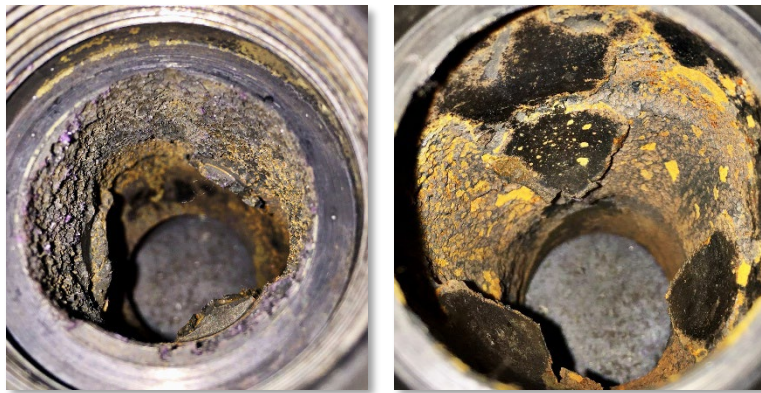
Figure 3 – Corrosion is another factor in metal cages, particularly hardlined cages. In the photo on the left, the base material corroded to the point where the lining completely separated from the body. These pieces of hardened material likely caused damage elsewhere in the pumping system. The photo on the right shows severe corrosion, but the hardened tabs are still present. The area around the ball has also corroded allowing the ball excessive lateral movement, which can indirectly result in ball and seat damage.
