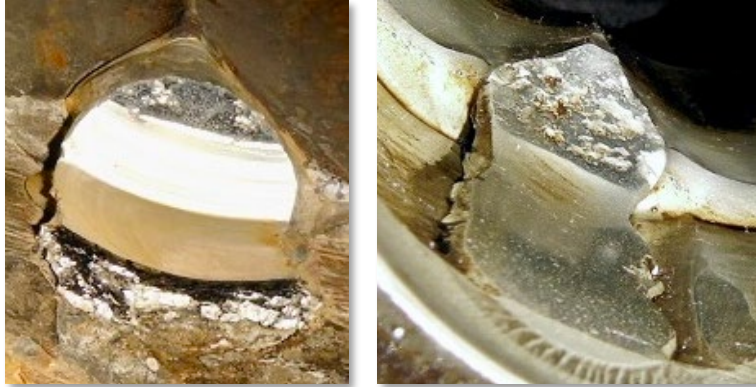
Figure 2 – The cages show above are severely beat-out. The chipping of the lining and undermining of the softer base material can be clearly seen around the edges of the lining face.
