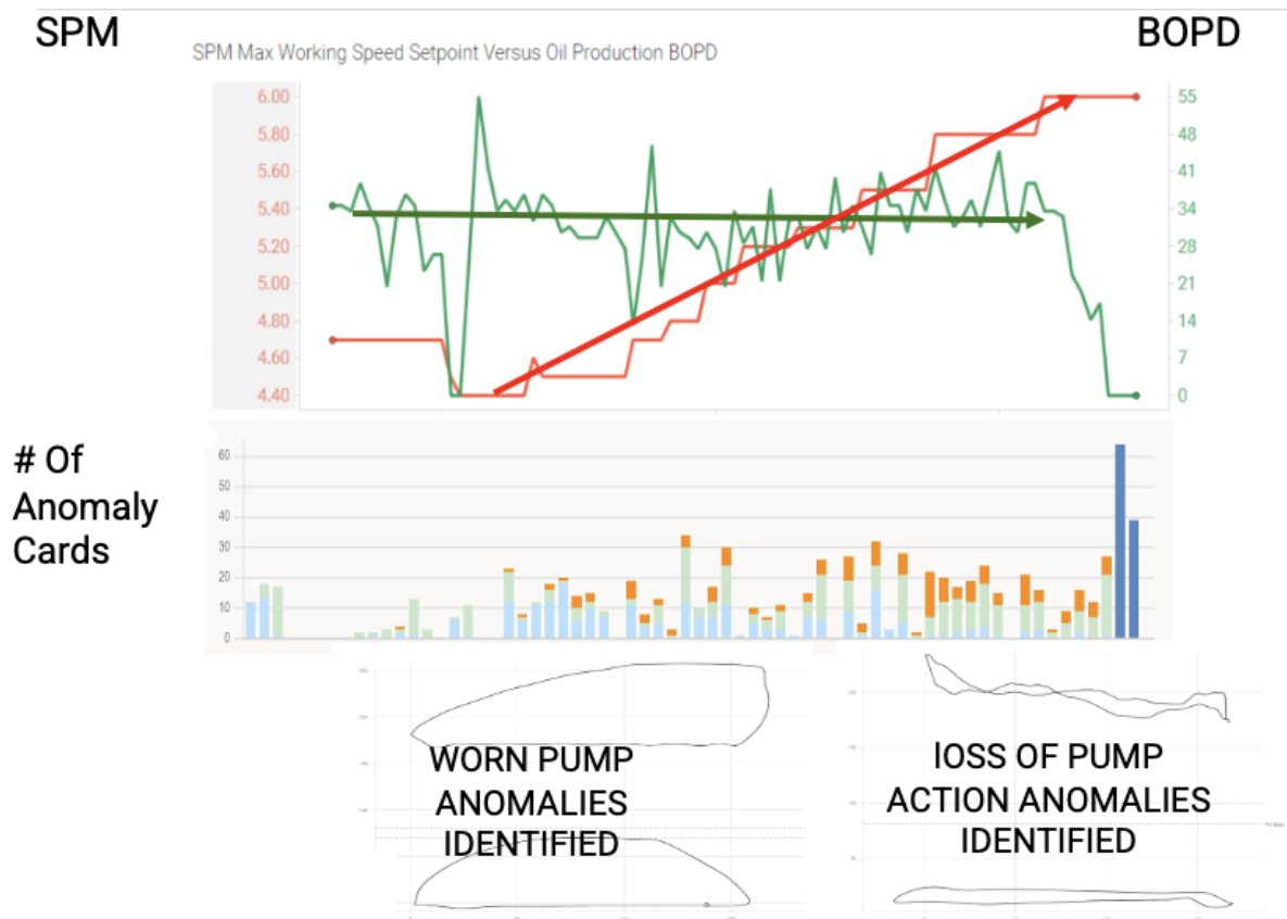
Figure 3 - CCR Working in Parallel with ASPM to Detect and Respond to a Worn Pump
