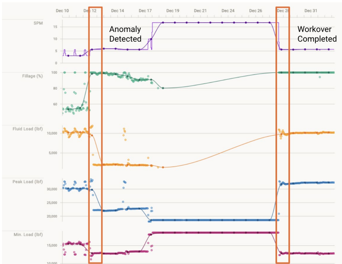
Figure 1 - Anomaly Detected 5 Days Prior to Failure
