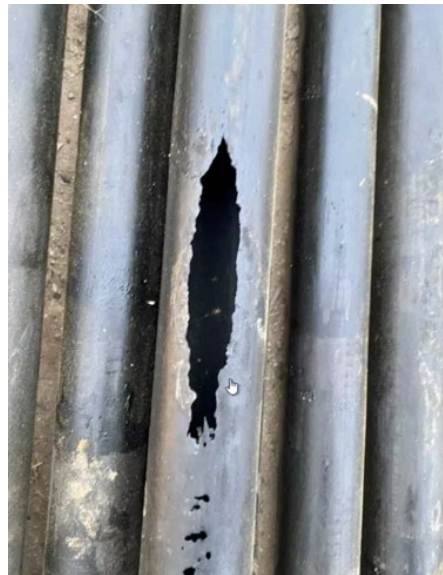
Figure 2. Sampling of Holes in Tubing
