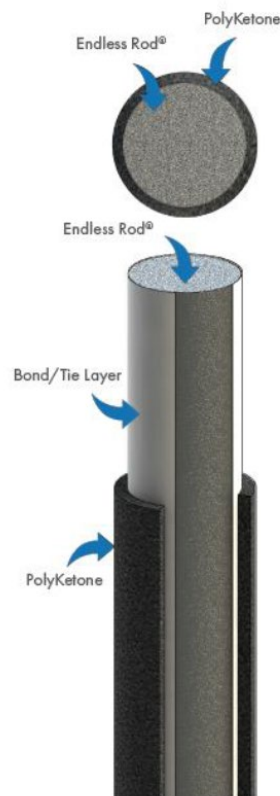
Figure 2. Cutaway diagram of coated continuous rod
