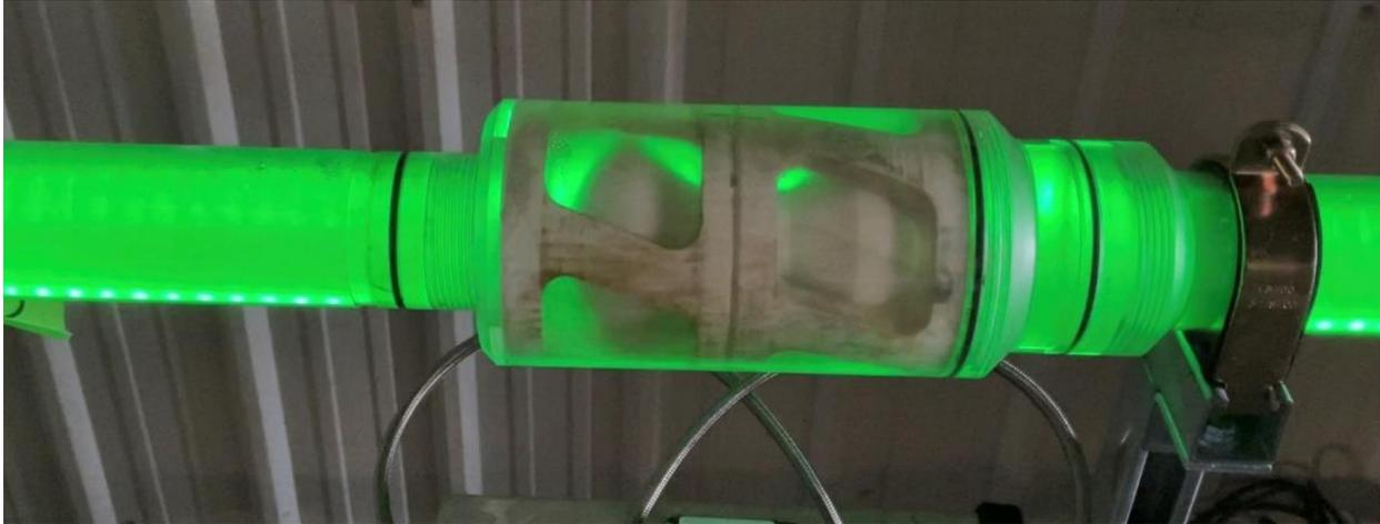
**FIGURE 24 – BARBELL FLOW LOOP TESTING PROVED VALVE FUNCTIONING BENEFICIALLY USES HYDRODYNAMIC FLOW DRAG**
