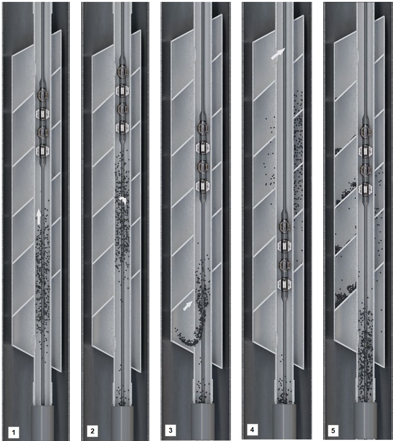
FIGURE 18 – SYSTEM PROCESS SEQUENCE OVER A FULL PUMP STROKE
