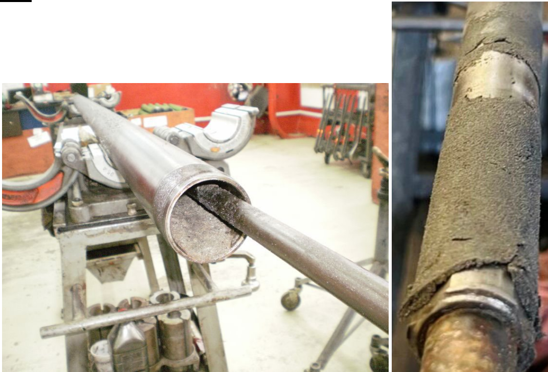
FIGURE 1 – SOLIDS ACCUMULATION IN AND ABOVE A SUCKER ROD PUMP, CAUSING A STUCK PUMP EVENT
