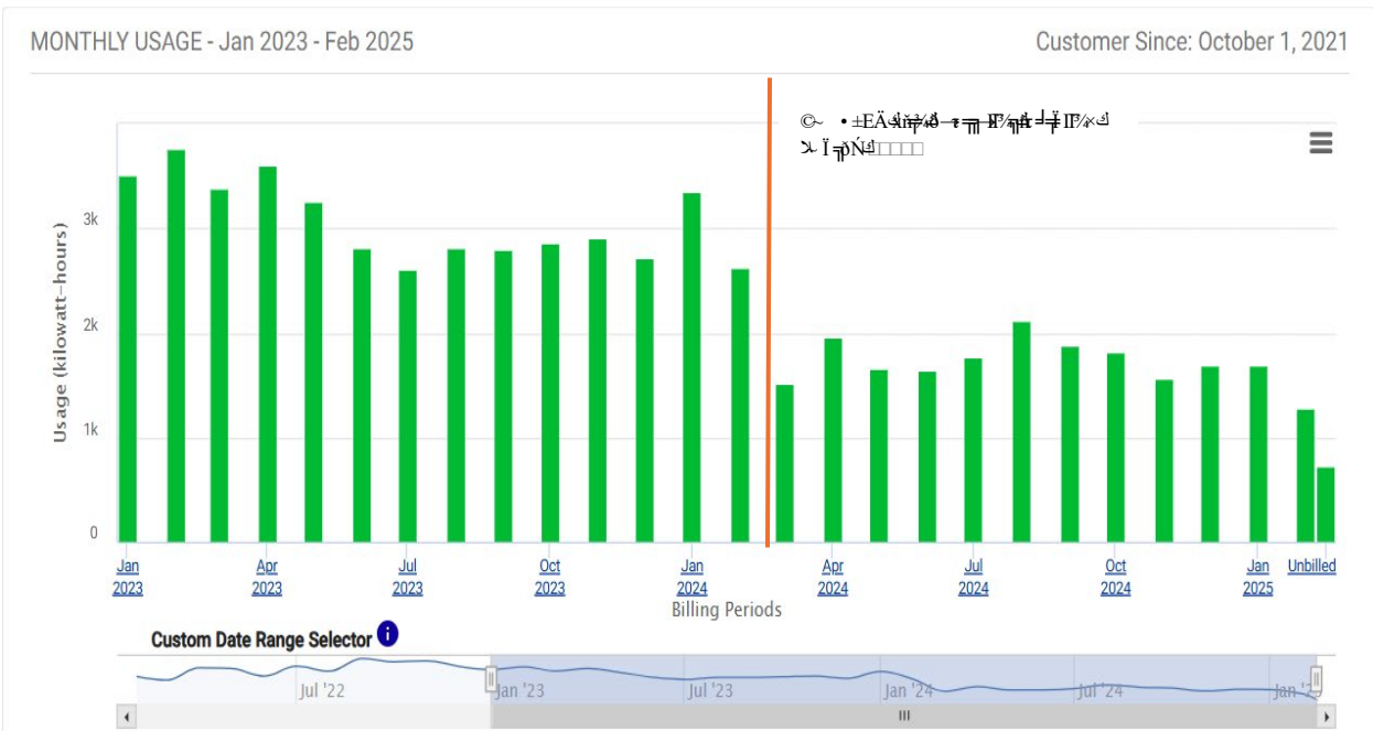
Figure 3 – The operator observed an average of 35% reduction in electrical costs.
