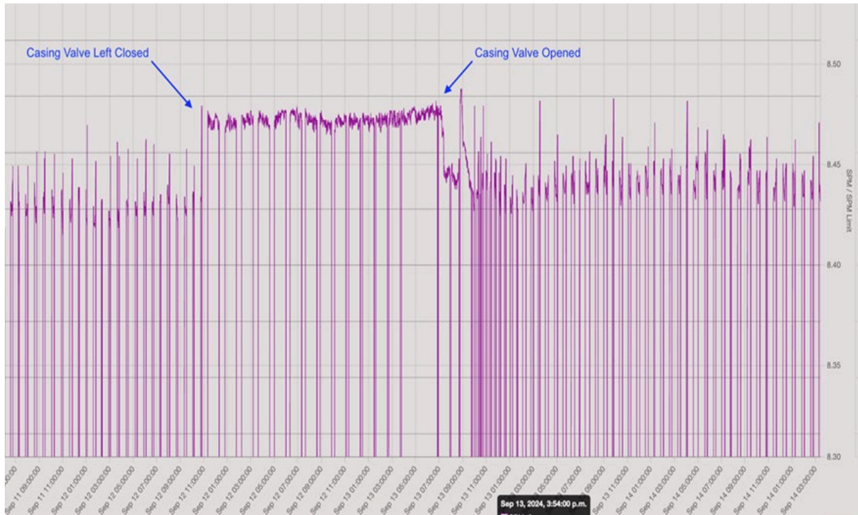
Figure 4 – Increased SPMs are seen when casing valve is left closed. A lighter fluid load is evident with closed casing valve; therefore, increased SPMs.
