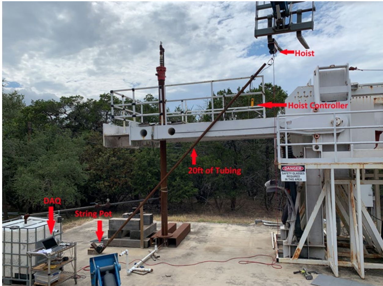
Figure 20 – ETA angled tubing test fixture that simulates deviated wellbores.
