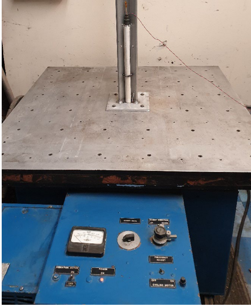
Figure 8 – Low frequency vibration testing of the DAS chassis assembly.
