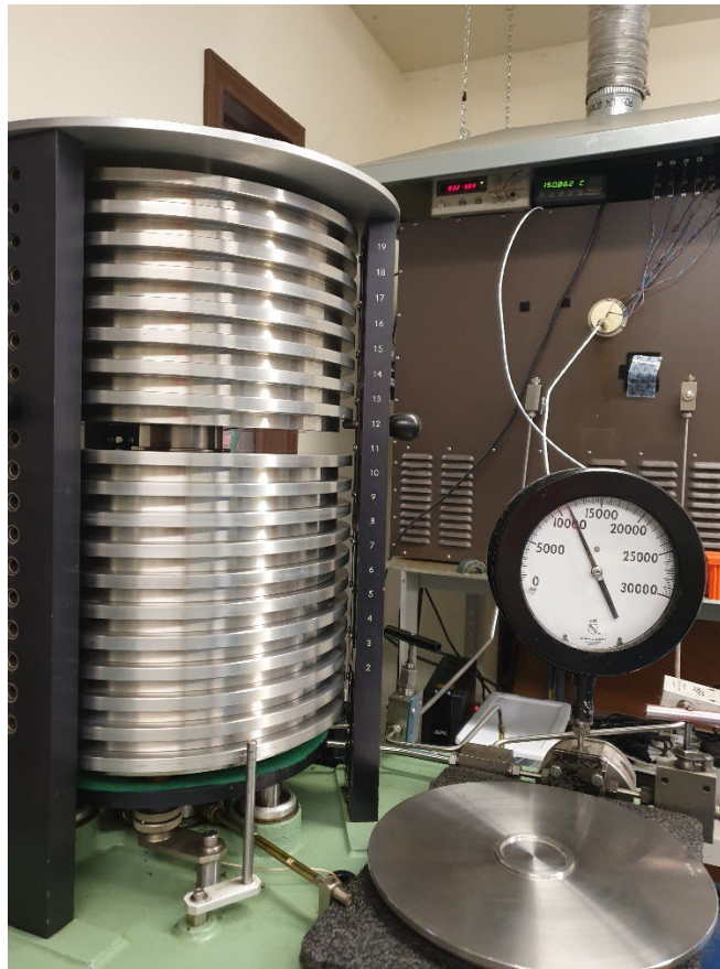
Figure 10 – Dead weight pressure standard used for pressure calibration.
