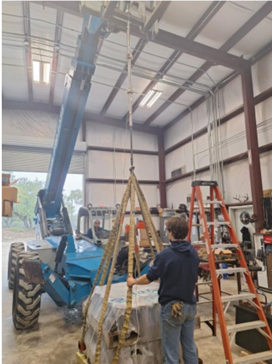
Figure 18 – Verification of load cell and load washer with 5250 lbm.
