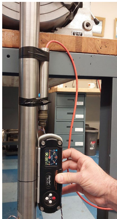
Figure 13 – Vertical tool alignment in rotary table using precision inclinometer.
