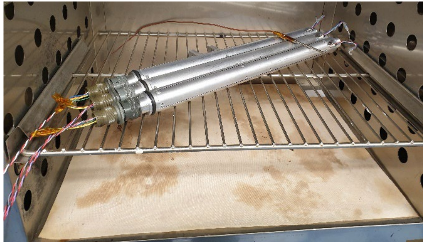
Figure 7 – Thermal testing of the DAS chassis assembly.
