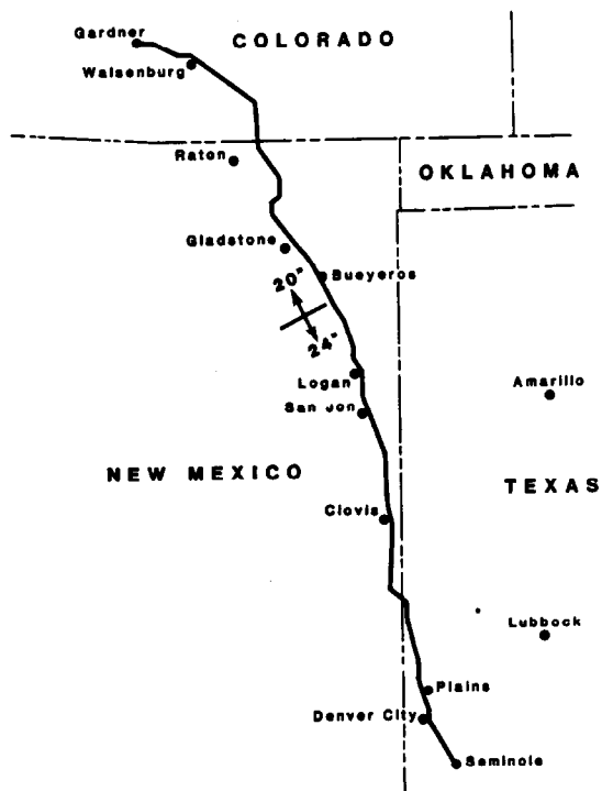
Figure 1 - Sheep Mountain Pipeline delivers CO 2 from Colorado to West Texas
