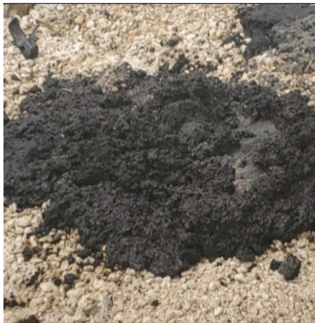
Figure 8- Sand found in the bottom mud joint.
