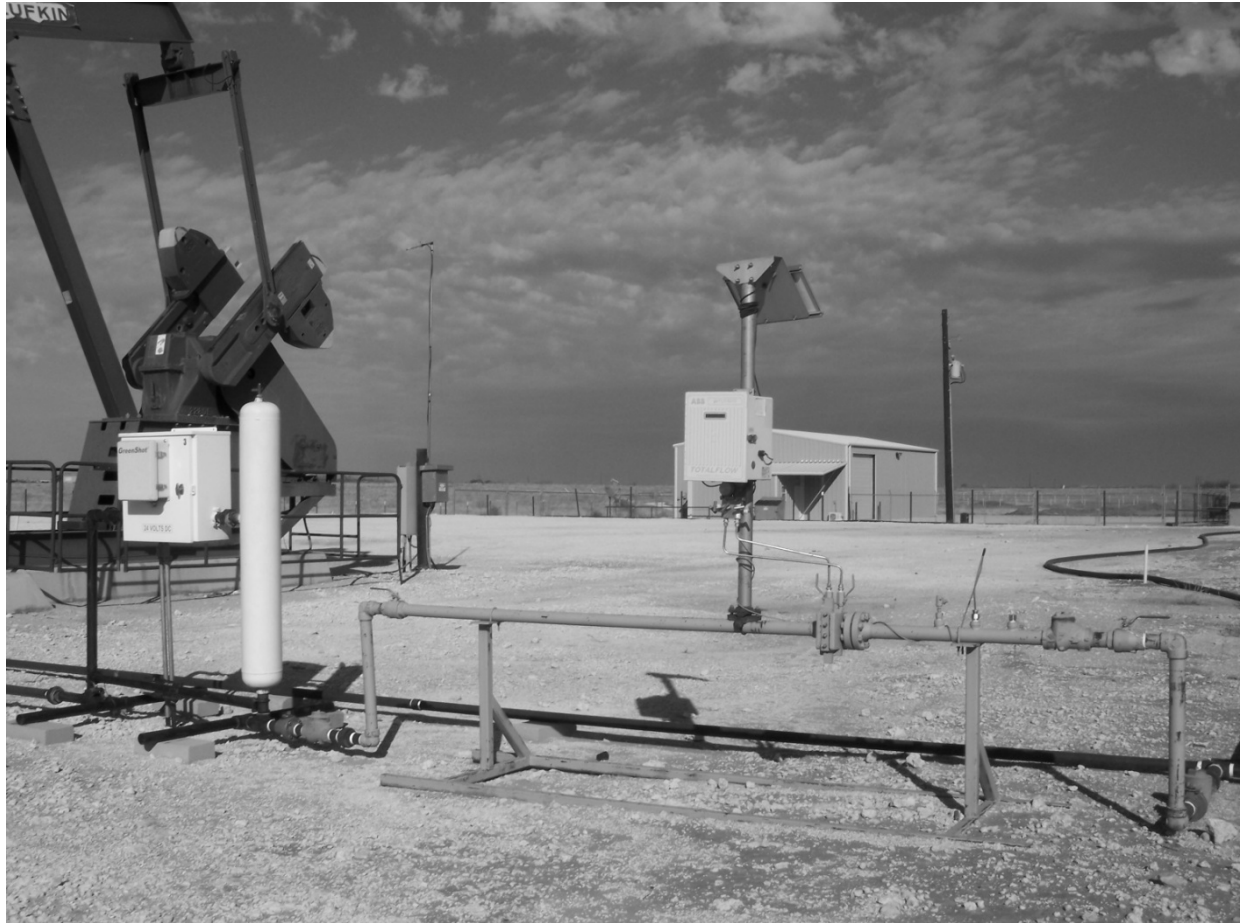
Figure 1 - New Device for Measuring Casing Gas and Green Fluid Level
