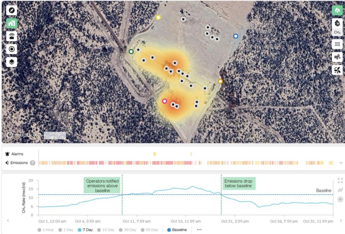
Figure 4 – Case Study 1: Regulator malfunction at a central tank battery and compressor station.
