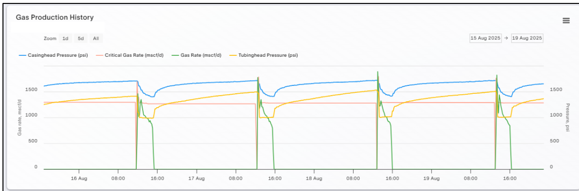
Figure 1 - Shut-in trigger logic: real gas rate versus critical gas rate with liquid loading onset
