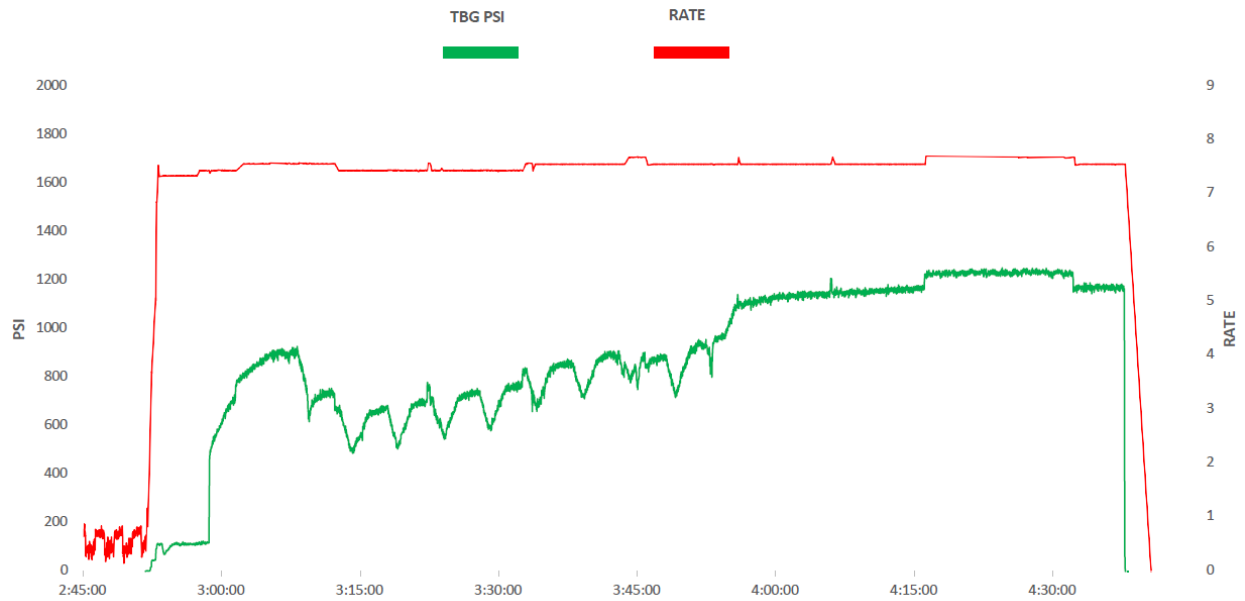
Graph 3. Diversion Performance for a 9-Stage Treatment with 267 lbs. of PLA per Stage
