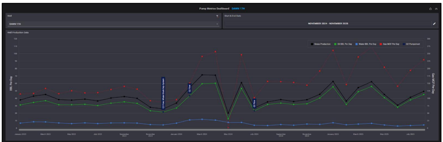
Figure 3: Pump Metrics Dashboard in Q2-Trak showing time-aligned oil, water, and gas production with pump history overlays for a single well.
