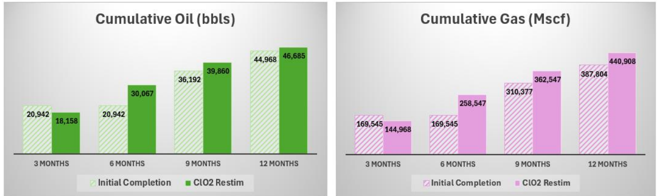
Figure 12: One Year Cumulative Production of Well R Post Original Completion (2015) & \text{ClO}_2 Treatment (2025).
