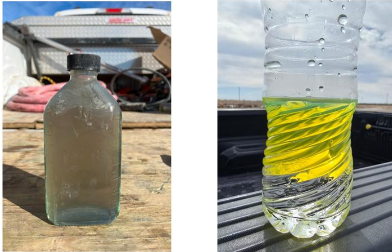
Figure 10: Flowback Fluid of Well R After 2 Days (Left) and 14 Days (Right) post ClO 2 Treatment.
