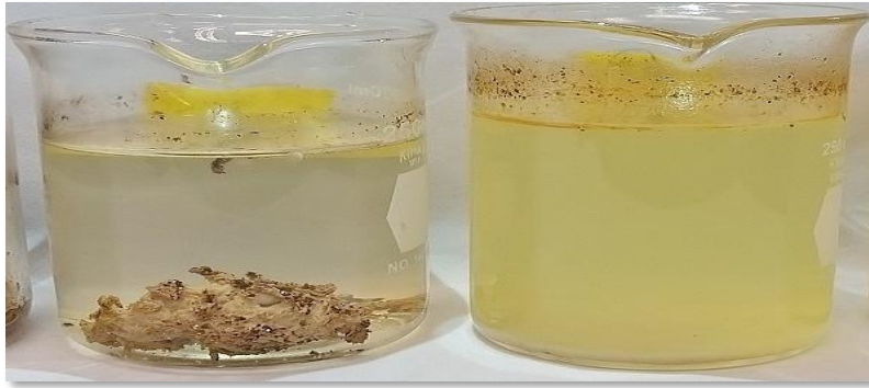
Figure 2: Solubilization of dehydrated guar gum residue using acidified Chlorine Dioxide (ClO 2 ).
