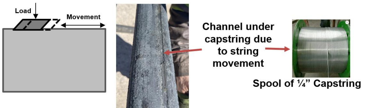
Figure 6: Fretting corrosion example.
