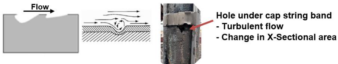
Figure 3: Erosion corrosion example.
