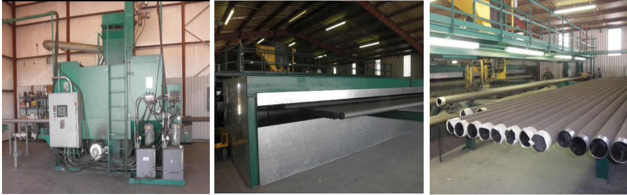
Figure 107: Grit blasting, curing process, and final product of epoxy resin coating.
