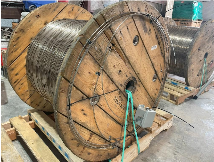
Figure 2. Fiber Optic Sampling Cable (2x10,000ft reels) w/testing box. Source: SLB/Geopsi
