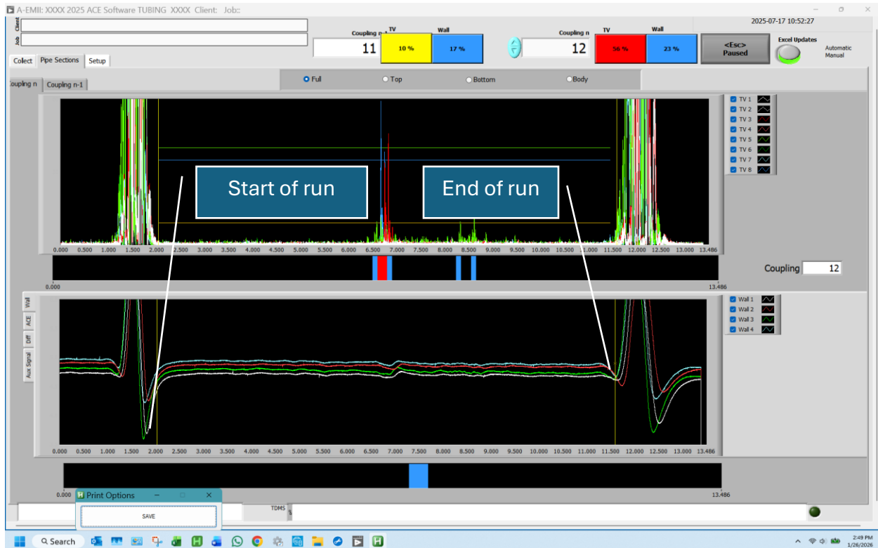
Generic graph showing the coupling pattern and point of reference identify by AI to start and end data evaluation.
