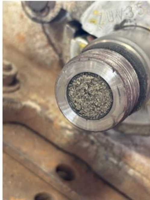
plunger packed off with sand
