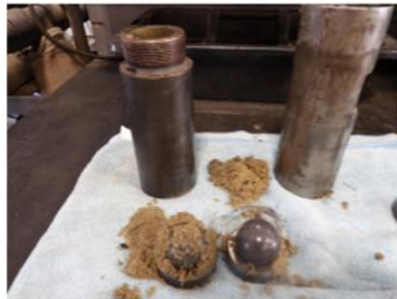
Standing valves prior to cleaning
