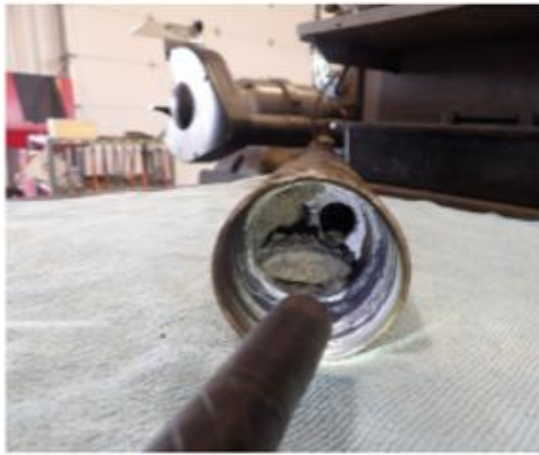
Sand in primary standing valve
