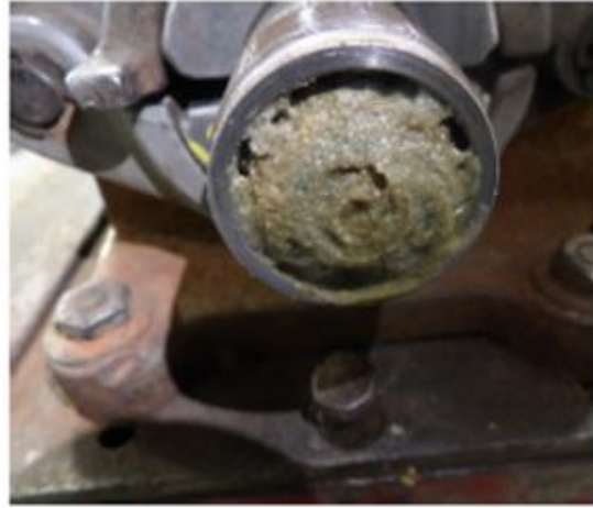
Barrel packed off sand
