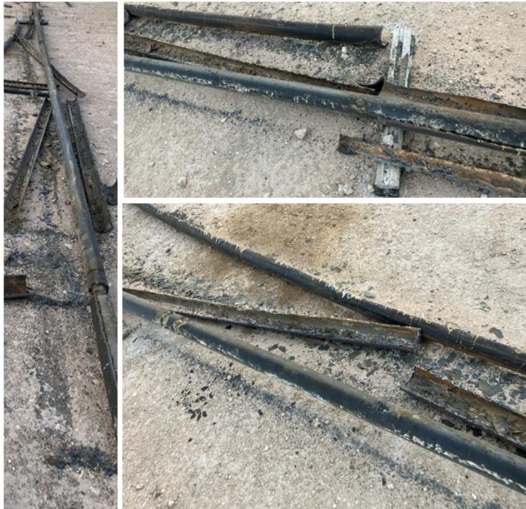
Figure 5. Equipment and the shroud after cutting.
