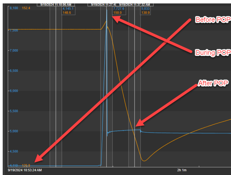
Figure 4: Pressure gauge data showing that the packer was able to hold ~1000 psi DP for multiple days. Plot shows BHP and temperature before and after the activation of the pump out plug.
