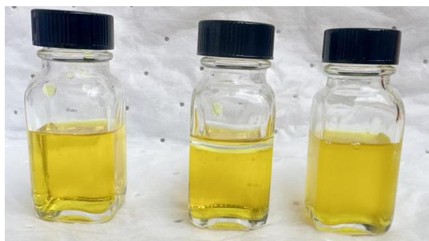
Fig 9. From left to right bottle with 15% HCl, 15% HCl with 10% xylene, and 15%HCl with 10% Multifunctional Formulation
