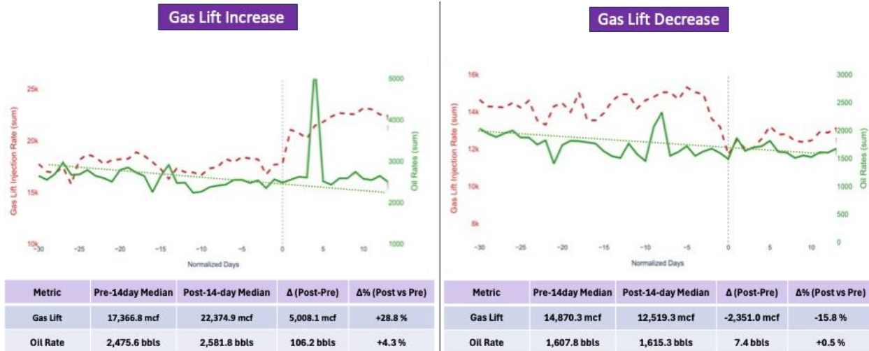
Figure 11 – Effect of implemented recommendations for gas lifted wells
