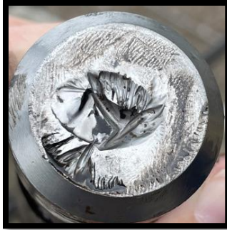
Figure 12 – 2-3/8” BHA Fishneck Damaged
