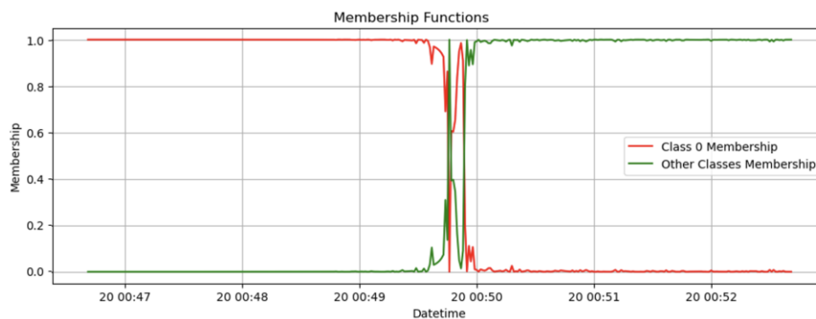
Figure 6. Fuzzy membership transformation of pressure signal for regime transition identification: Example 2. Source: SLB
