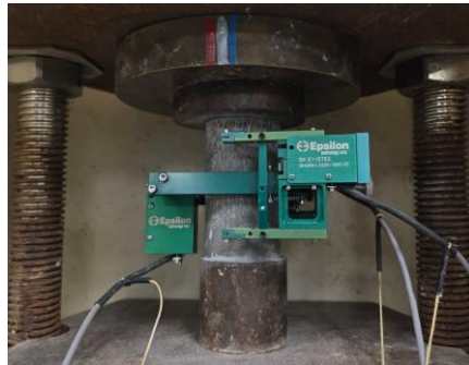
Figure 11 - Uniaxial Compression Test Setup with Epsilon Extensometer for Stress-Strain Measurement
