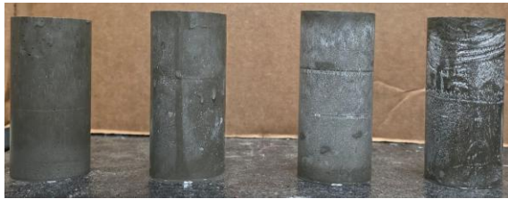
Figure 12 - 13.7 ppg Neat Class C Specimens (Left to Right: 0%,10%,20%,30% Resin)
