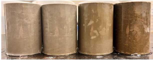
Figure 14 - 14.8 ppg Neat Class C Specimens (Left to Right: 0%,10%,20%,30% Resin)
