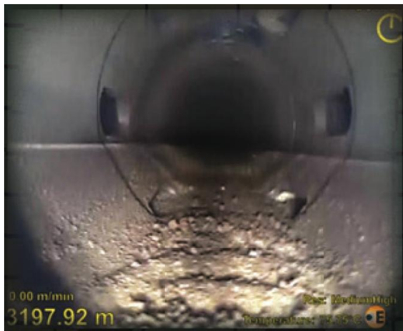
FIGURE 10 – SOLIDS DUNE/BED MIGRATION ACCUMULATION NEAR THE BASE OF THE WELLBORE'S CURVE SECTION
