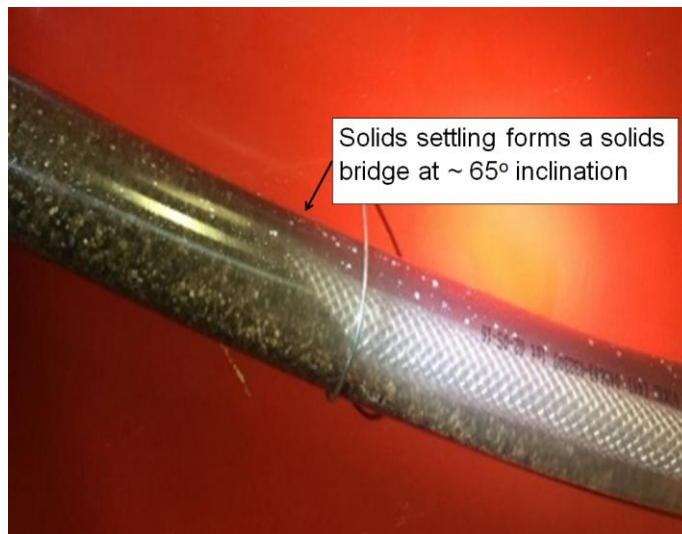
FIGURE 9 – SOLIDS SETTLING ANGLE OF REPOSE IS 65 DEGREES FOR TYPICAL SOLIDS PARTICLE SIZES EXPERIENCED FOR ROD PUMPING
