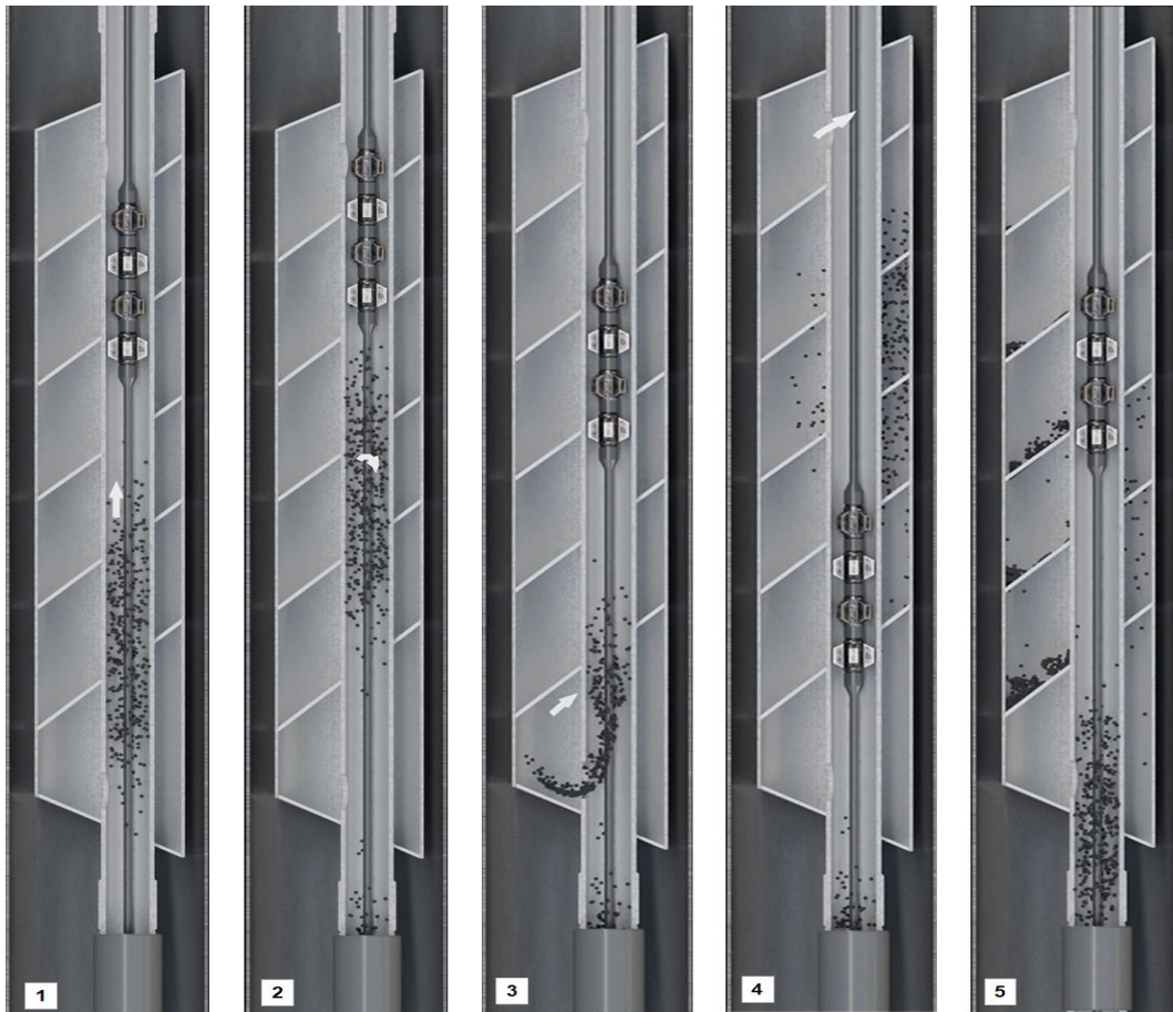
FIGURE 35 – SANDSHARK TOOL'S SOLIDS SEPARATION ASYMMETRIC MULTI-STAGE WEIRS AND CHANNELS THREE-DIMENSIONAL RENDERING
