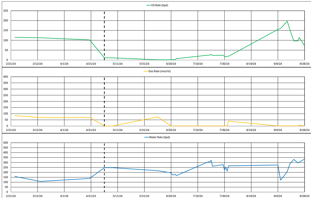
Figure 1C: Well C - Oil, gas, and water production rates versus time prior to surfactant application with the vertical dashed-line indicating the frac-hit event.
