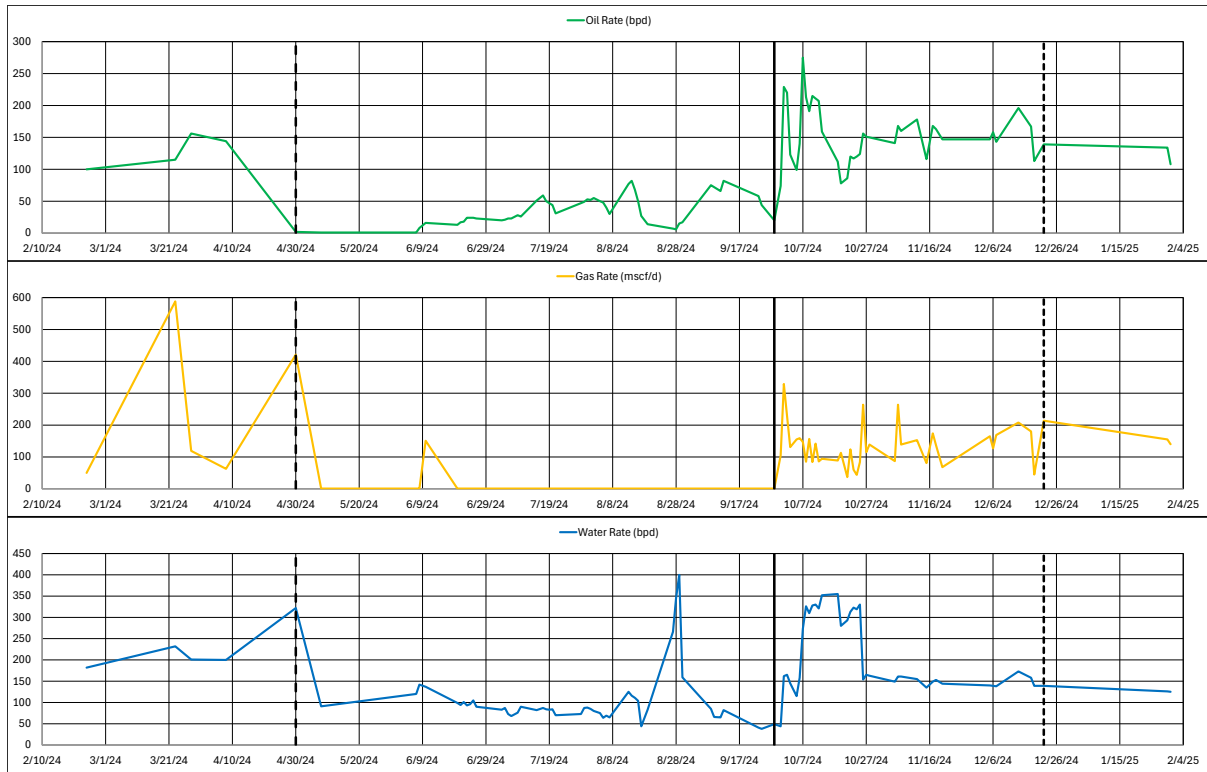
Figure 2A: Well A - Oil, gas, and water production rates versus time before and after surfactant application.
