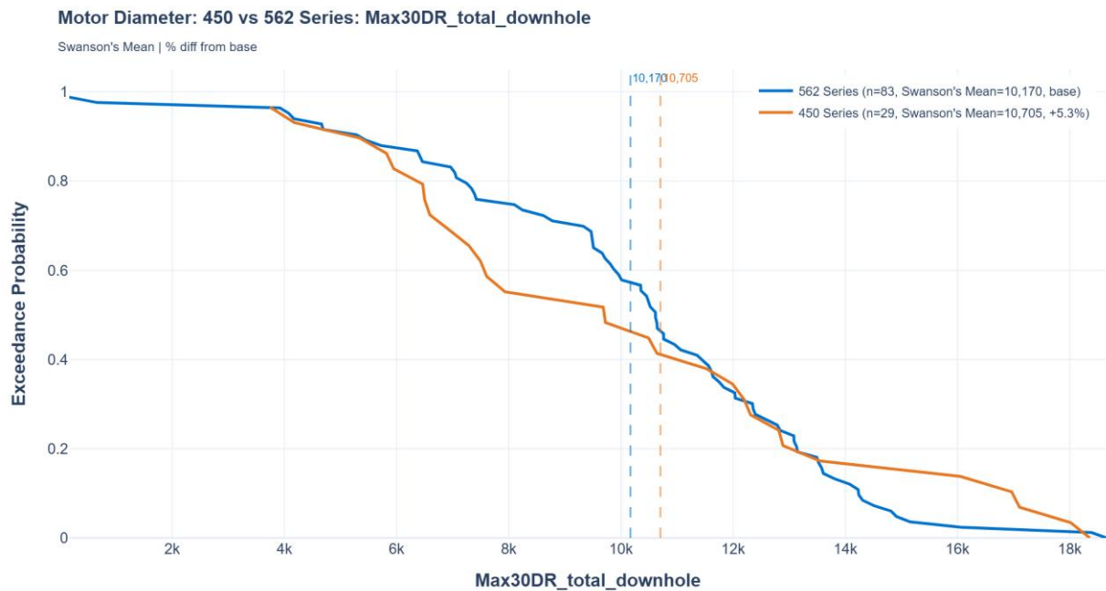
Figure 11 - Downhole produced volumes between 450-series and 562-series motors in 7.625 inch casing with 1,750 and 2,000 BEP pumps
