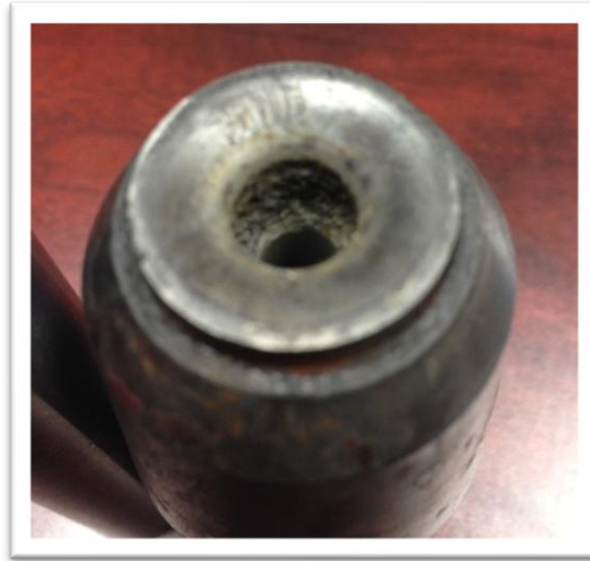
Figure 11: Production Cavitation Damage on a Jet Pump Mixing Tube
