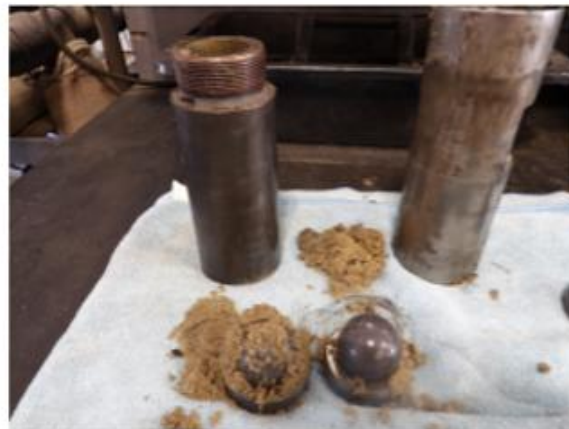
Standing valves prior to cleaning
