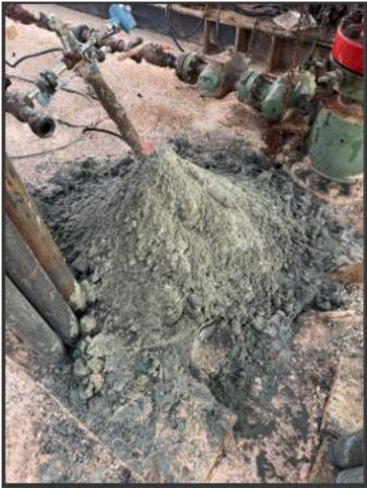
Figure 2: Examples of solids found during the pulls and pump teardowns.
