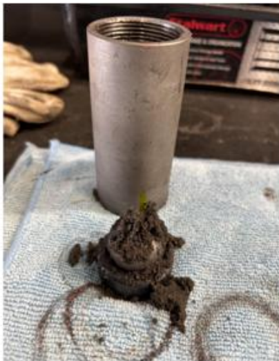
primary traveling valve ball and seat
