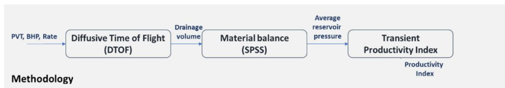
Figure 1 – Transient well performance modeling scheme (Parekh, Zalavadia et al. 2025)
