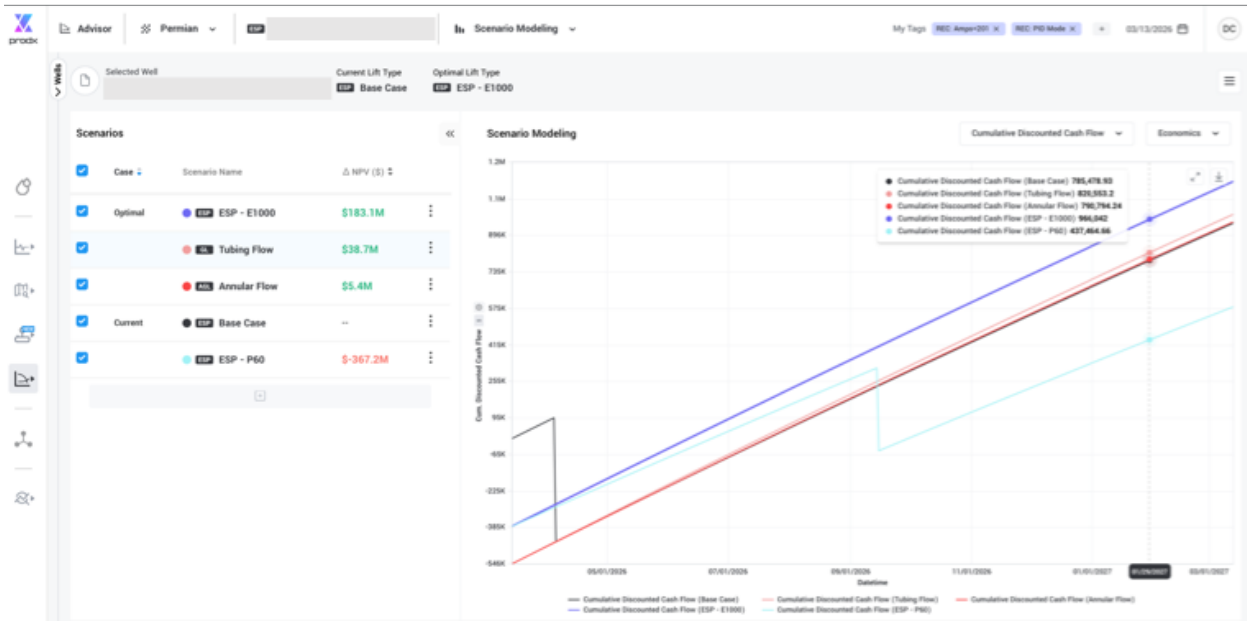
Figure 24 – Forecasted revenue for different artificial lift scenarios for the example wells.
