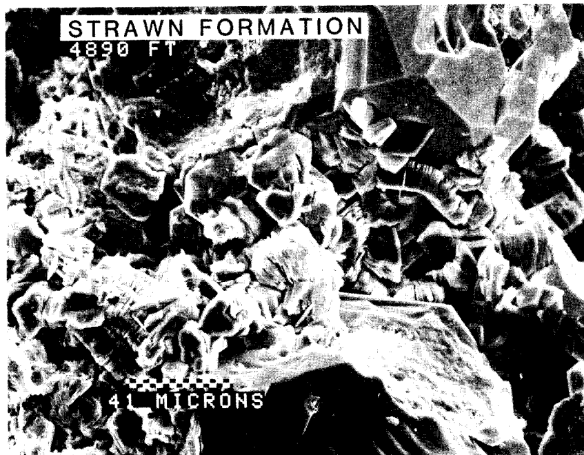
Figure 4 - Electron micrograph of an enlarged portion of Figure 3. The large, well-formed crystal faces of quartz grains (Q) suggests that an authigenic regrowth of quartz has taken place. Authigenic kaolinite clay can be seen bridging the intergranular void between quartz grains. Magnified 490 times.
