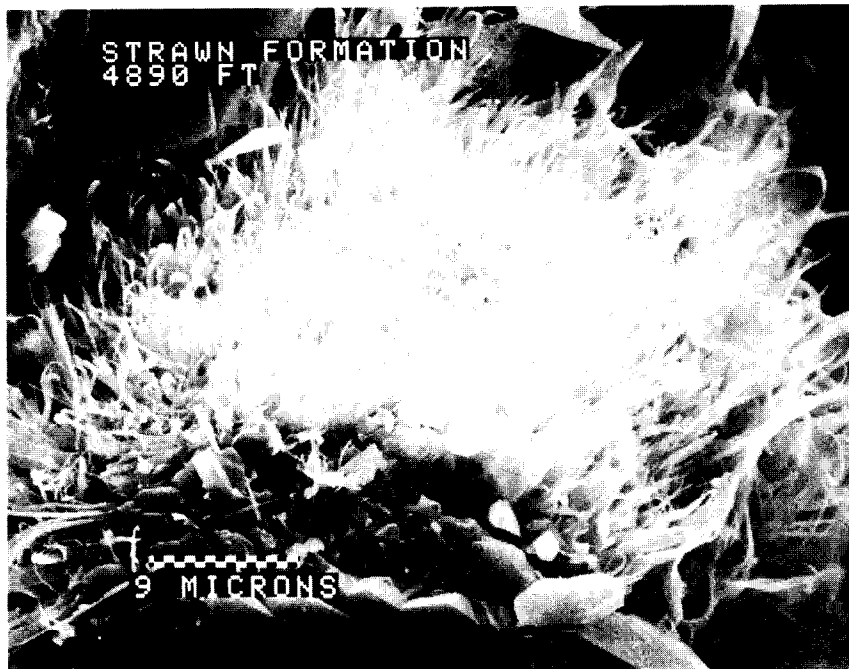
Figure 6 - Scanning electron micrograph of an isolated aggregate of illitic clay. Note the distinctive filamentous appearance. Magnified 2500 times.
