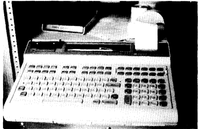
FIGURE 4—HEWLETT-PACKARD SIGNAL CONVERTING COMPUTER. THE COMPUTER ACCEPTED DATA TYPED IN ON THIS CONSOLE. INSTRUCTIONS FOR DATA PRESENTATION AND VARIATIONS OF TIME BETWEEN DATA PRINTINGS WERE GIVEN TO THE COMPUTER.
