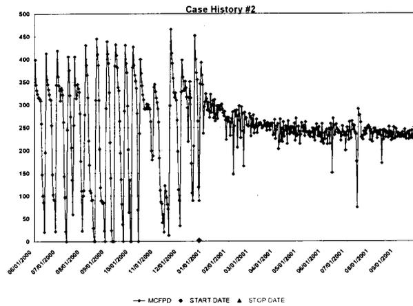
Figure 5 - Capillary Installation to Stabilize Production
