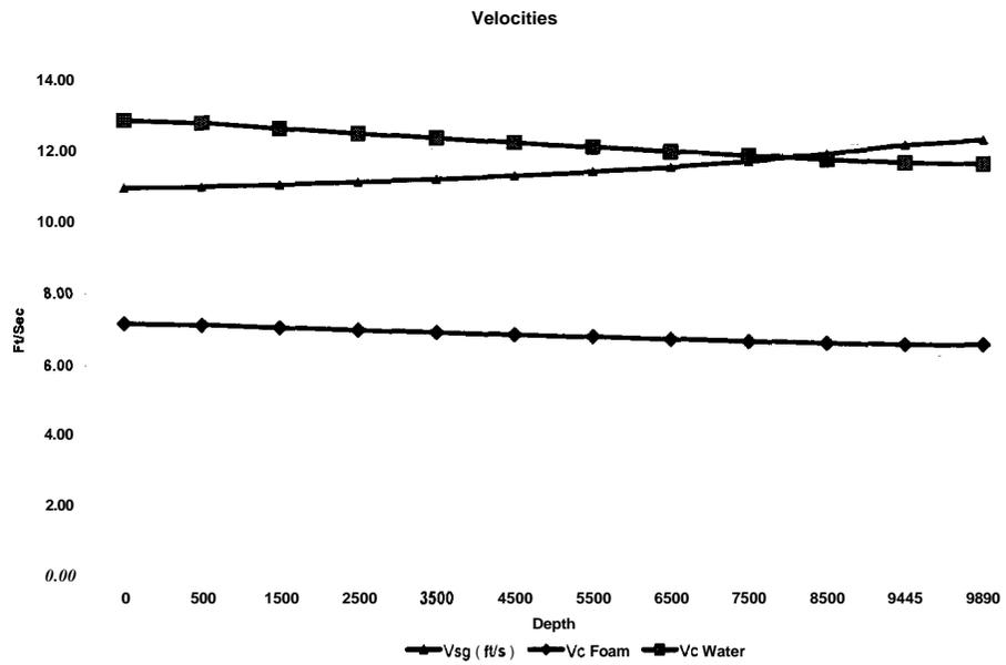
Figure 3 - Velocity Distributions from Perfoam™ Model
