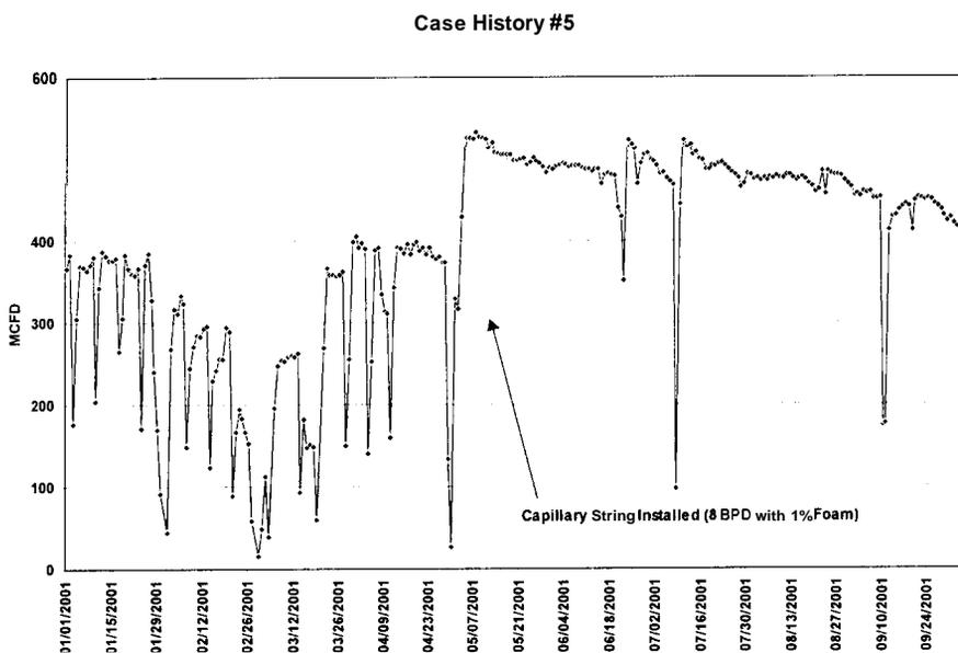
Figure 8 - Capillary String Remove Salt Deposition
