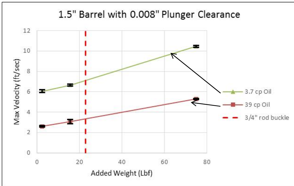
Figure 6 Maximum Plunger Velocities for the 1.5" pump with 0.008" plunger clearance.
