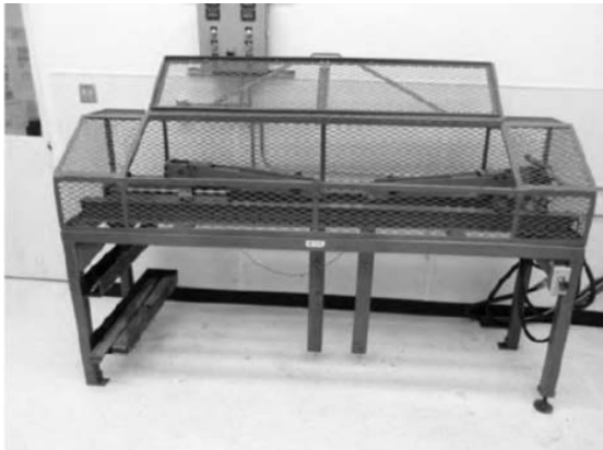
Fig 10. Small rotary bend fatigue tester
