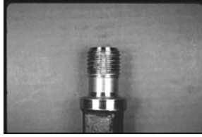
Figure 13 - Improper Lubrication Damage
