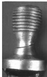
Figure 10-Pin Damage Due To Excessive Makeup Torsion
