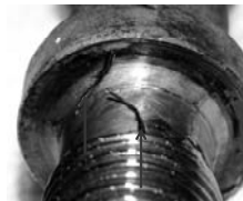
Figure 4 - Damage from Knocking Off Protectors
