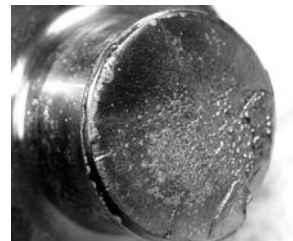
Figure 12 - Excessive Torsion Damage
