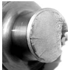
Figure 15 - Loss Of Displacement Failure
