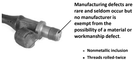
Figure 1 - Manufacturing Discontinuities or Defects
