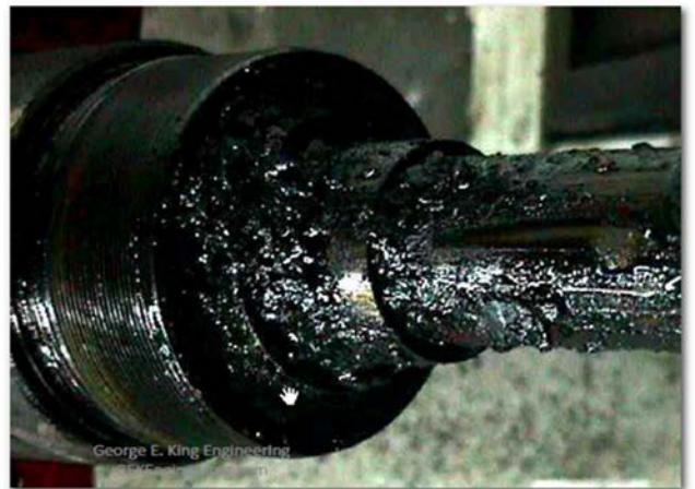
Figure 4. Asphaltene Coated Tubing
