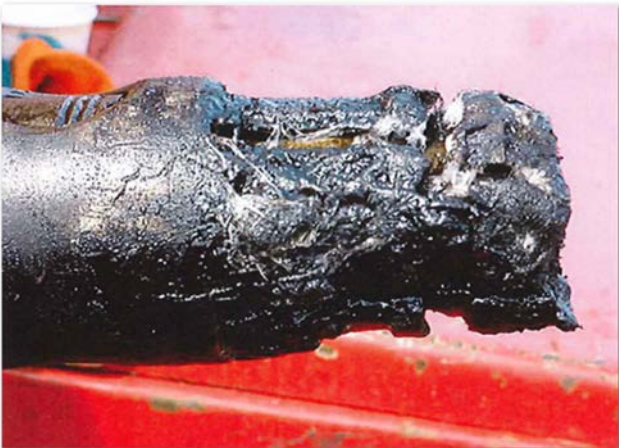
Figure 3. Asphaltene Coated Slickline
