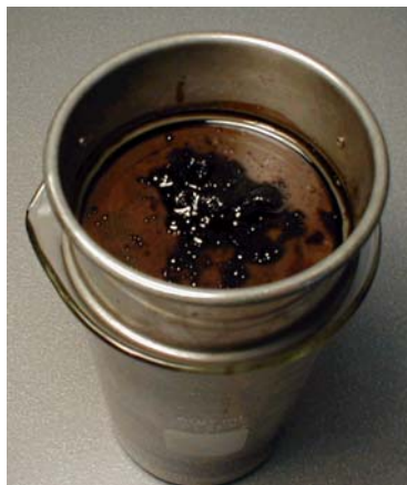
Figure 7 – Illustration of acid sludge from San Andres oil and 15% Hydrochloric Acid.
