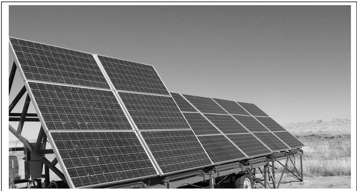
Adjusting panels to the winter angle for more direct sunlight
