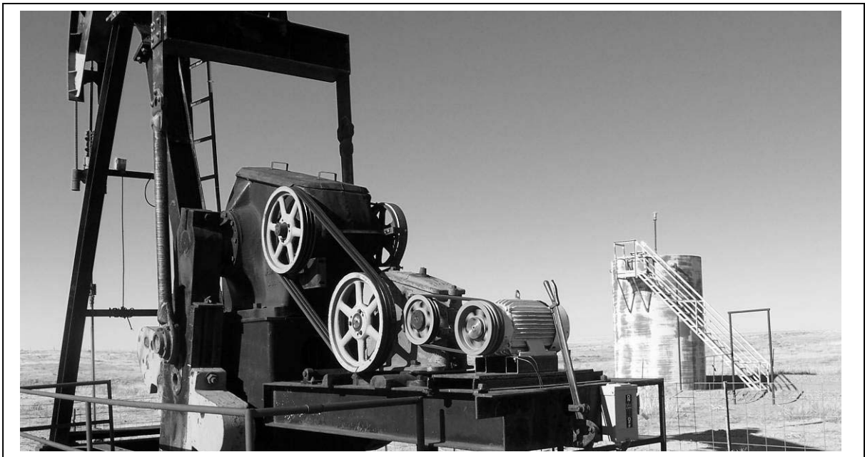
Installation of 10HP 220 VAC, 3 phase motor (Actual power requirement uses 2.2HP)
