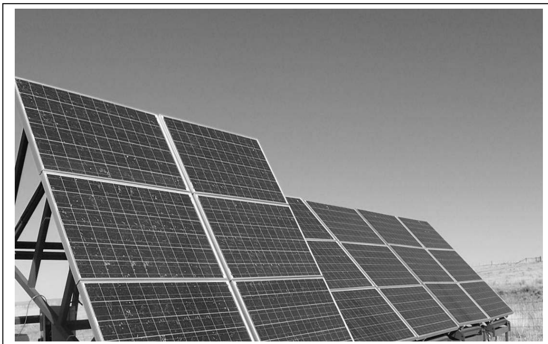
ADJUSTING SOLAR PANELS TO WINTER SUN ANGLE
