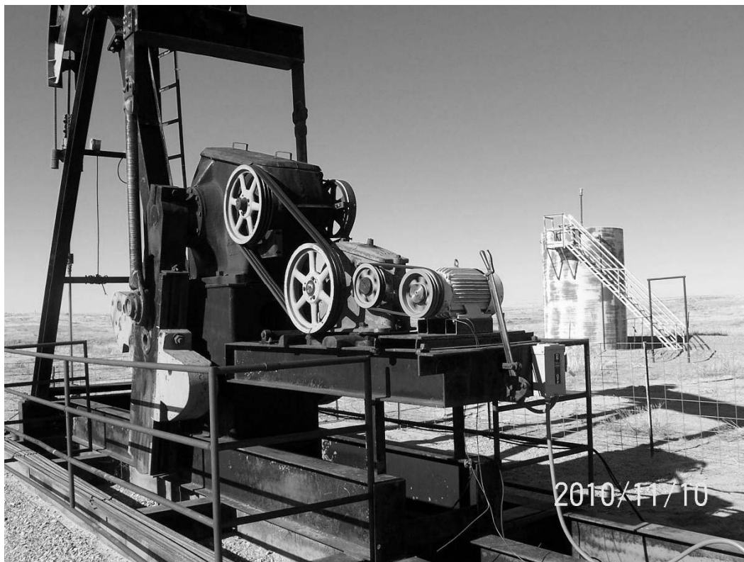
INSTALLATION OF 10 HP 220 VAC, 3 PHASE MOTOR WITH ACTUAL PUMP POWER REQUIREMENT OF LESS THAN 3 HP.
