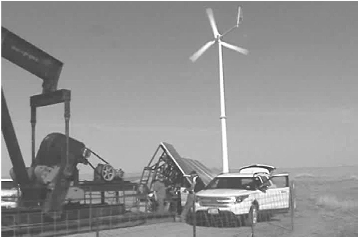
5 KW WIND TURBINE WORKING IN CONJUNCTION WITH 3 KW SOLAR PANELS
