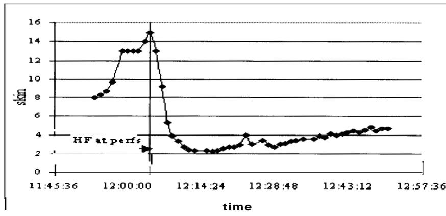
Figure 7 - Gradual Damage Caused by Excessive Acid Injection
