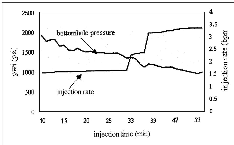
Figure 5 - Flow Rate and Bottomhole Pressure for Sandstone Acidizing Treatment
