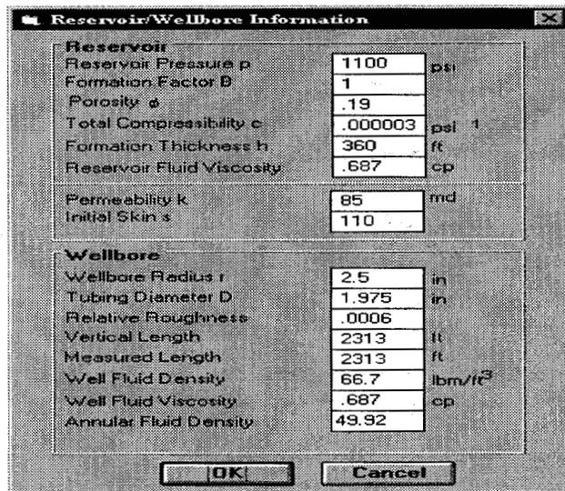
Figure 3 - The Reservoir/Wellbore Information Panel for Vertical Well
