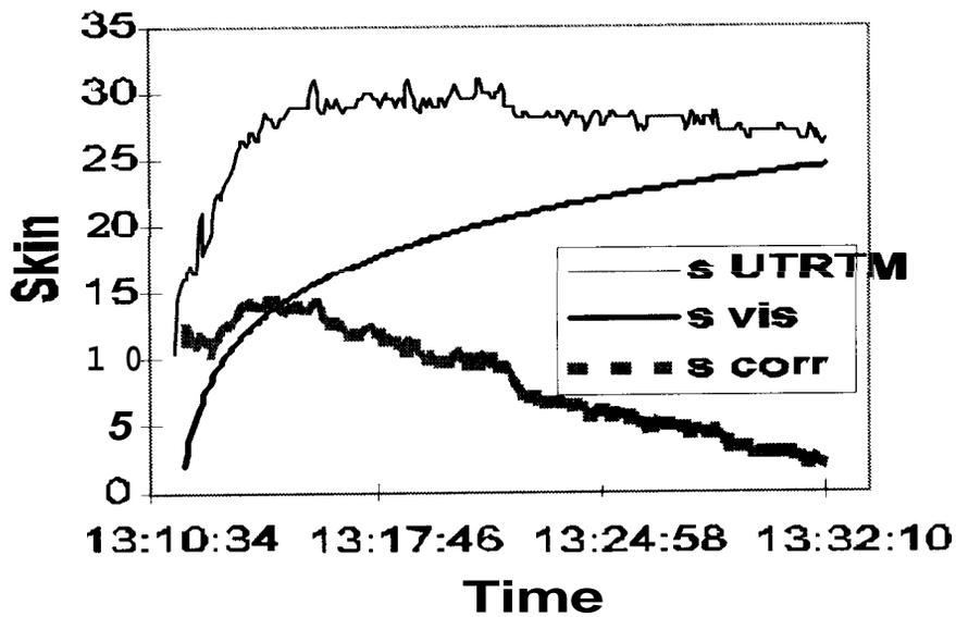
Figure 10 - Skin Factor Response of a Gas Well Illustrating Viscous Skin Effect
