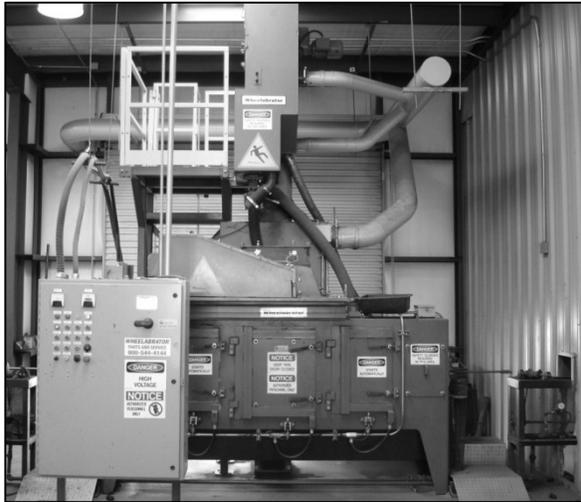
Figure 1 – sucker rod shot peening machine
