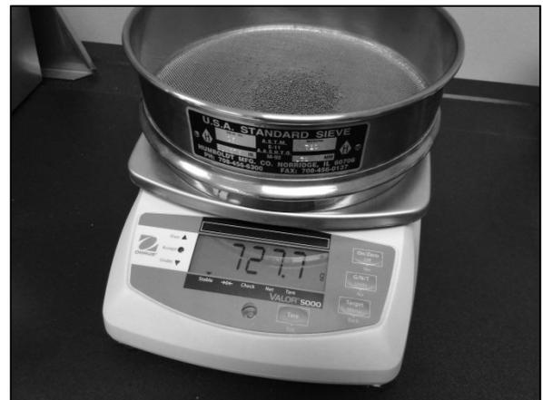
Figure 10 – digital scale for weighing screened samples
