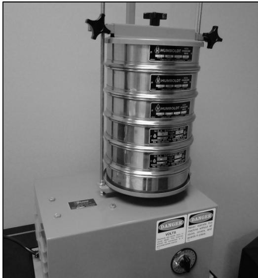
Figure 9 – sieve screening for particle size analysis
