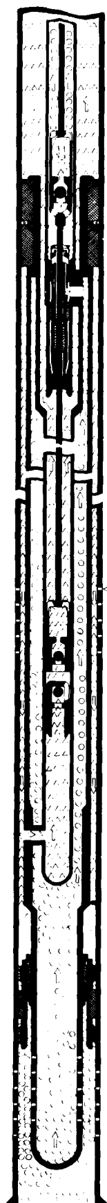
SCHEMATIC DIAGRAM OF DOUBLE CROSS-OVER ASSEMBLY SHOWING FLUID FLOW.
