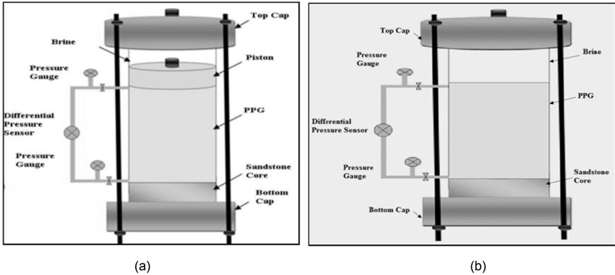
Figure 1 - Gel Pack Schematic a) Model I b) Model II
