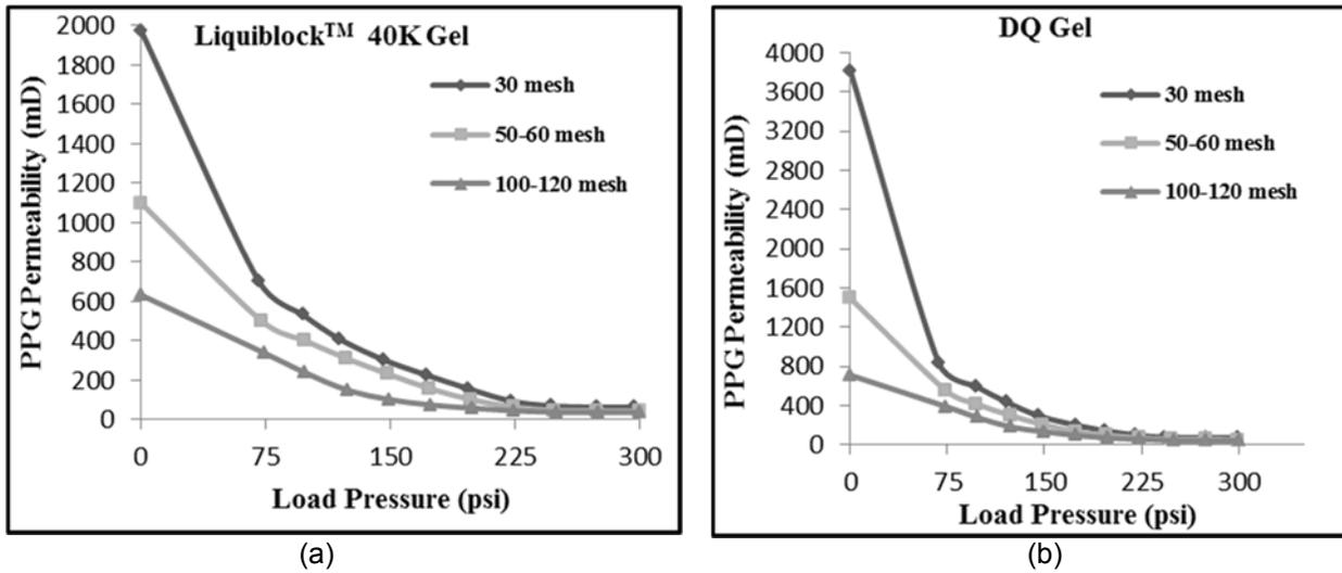
Figure 4 - The effect of load pressure on PPG pack permeability for various particle sizes of a) Liquiblock™40K gel, and b) DQ gel.
