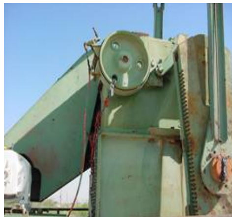
Chain and Binder Properly Placed on Break Drum
