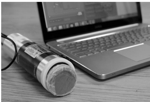
Figure 1- Overview of Gamma-ray Spectrometer, NaI(Tl) and 20 gram sample.
